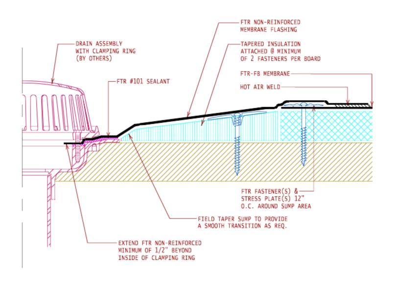
NOTE: USE TAPERED ROOF INSULATION (EDGE STRIPS) TO CREATE DRAIN SUMP. IF TOTAL INSULATION THICKNESS IS LESS THAN OR EQUAL TO 1 1/2 IN., TAPER 12 IN. FROM THE DRAIN CENTER. IF TOTAL INSULATION THICKNESS IS GREATER THAN 1 1/2 IN., TAPER 18 IN. FROM DRAIN CENTER.
