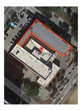
The Work of this Specification includes the roof area known as the "Seventies" building, located on the North. At three core sample locations, the roof assembly consisted of one layer of mineral granule surfaced built up roofing over inch and a half (1 1/2") polyisocyanurate insulation over a structural concrete deck. Core samples may not be representative of the existing roofing system at repairs or other areas.
