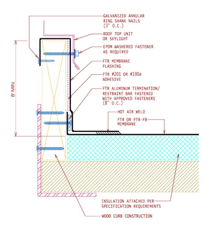
ROOF ACCESS HATCH / EXHAUST FAN CURB
