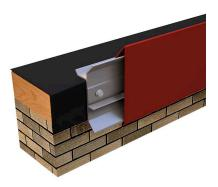
At lower level parapet walls, secure 2 x 8 wood nailer, cut to fit the angle at the outside edge, and cut the inner edge parallel to match. Apply 24 gauge clad metal using galvanized annular ring shank nails staggered six (6) inches on center, over 20 gauge continuous cleat, fastened three (3) inches on center. Use galvanized annular ring shank nails. Nails to have minimum one (1) inch penetration into wood.
